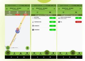
EPILOT 4.0 is managed with a dedicated Application where it is possible to monitor the system data and its correct functioning, the new features are the automatic ignition thanks to the integrated GPS and the variation of the quantity of hydrogen produced based on the speed in order to further improve consumption.
